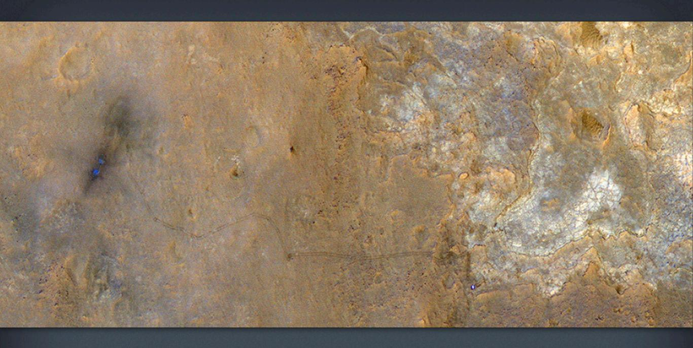
A Unique View of Curiosity Rover in Yellowknife Bay With enhanced colors, we can view the region around the landing site and Yellowknife Bay. The rover is the very bright spot near the lower right. The rover tracks stand out clearly in this view, extending west to the landing site where two bright, relatively blue spots indicate where MSL's landing jets cleared off the redder surface dust.
